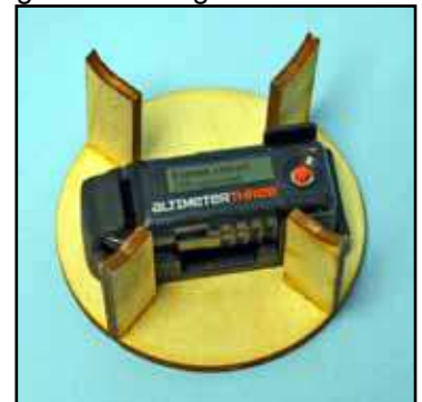
Figure 5: The altimeter mount for my egglofter.
